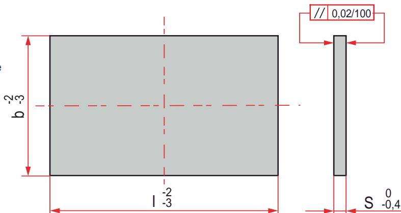
$$= 0,28 \text{ P} = 330 \text{ N/mm}^2 \text{ T máx.} = 240^\circ\text{C}$$
